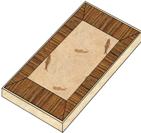
Figure 3-2: Contrasting Edges Shown on Face
